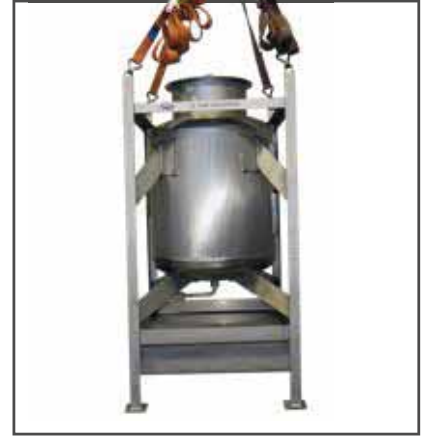
Top Lift Test
